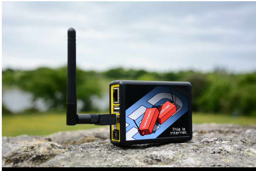
Figure: Internet Cube project, based on Olimex hardware and Yunohost software
